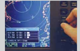
Dedicated rotary knobs to adjust GAIN/STC/FTC for simplified control.
