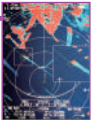
Target A3: Zoom box tracks the targeted object according to its movement
